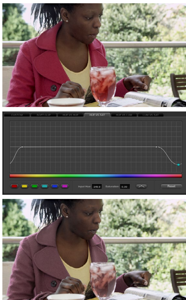
Lowering the saturation of the woman's jacket using the Hue vs. Sat curve; Top—original image, Bottom—altered image
