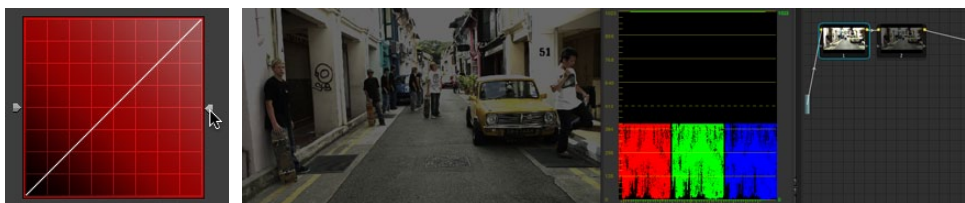
Lowering the High Clip slider in node 1 forces all image data above the new High Clip threshold to be irretrievably discarded. Clipped data cannot be brought back by subsequent nodes.
