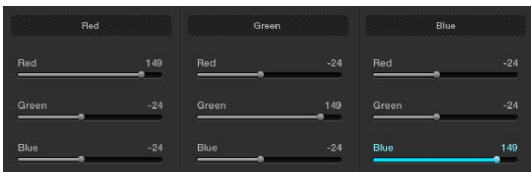
RGB Mixer settings used to boost saturation and reduce color channel crosstalk
