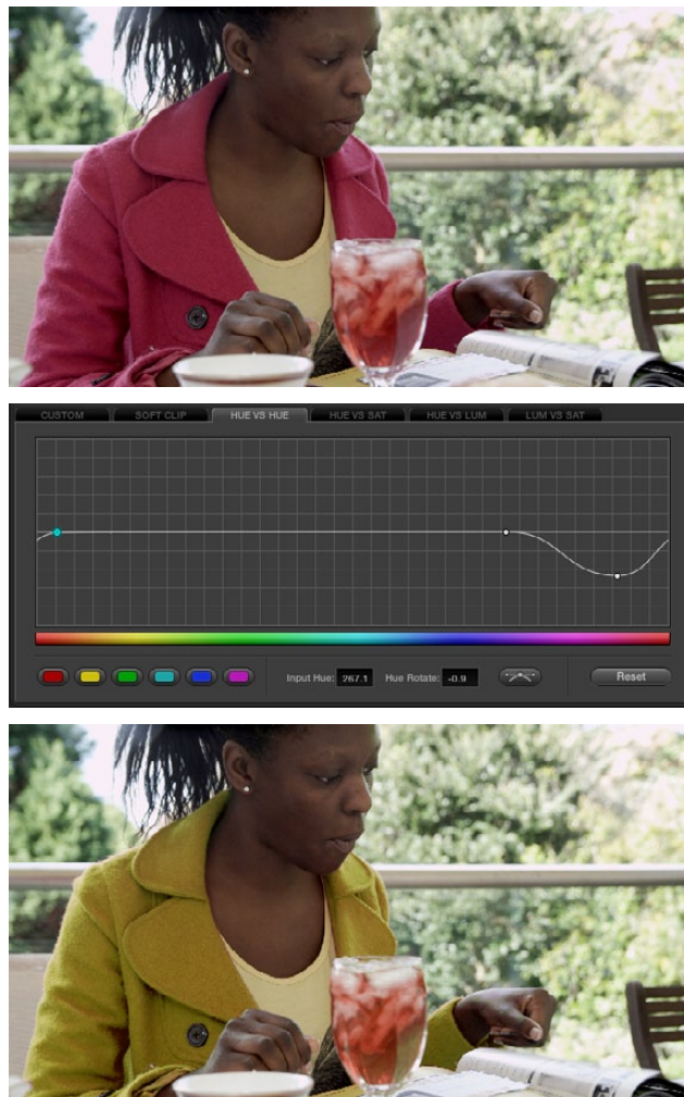
Top—Original image, Bottom— the image as altered by the Hue vs. Sat curve shown in the middle
