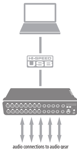
Figure 5-1: Using the Stage-B16 as an audio interface.
